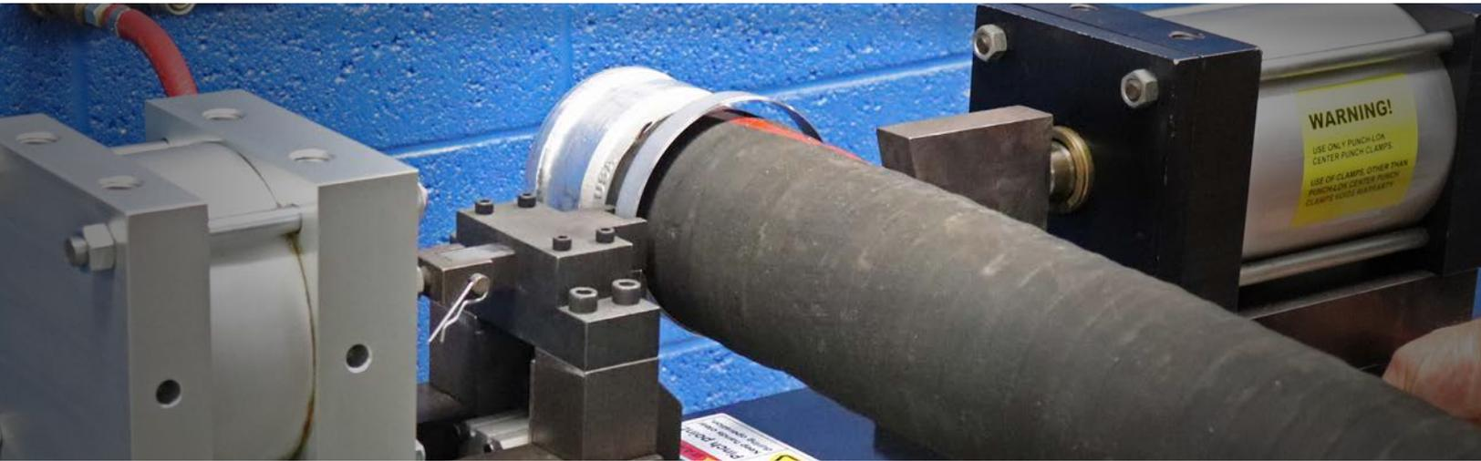
TENSION-AIR™ (TA-3 PLUS™) production hose clamping machines are entirely automatic. Developed by Punch-Lok®, our hose clamping machines eliminate the need for manual punching or bending when applying hose clamps to hose assemblies. Only requiring one person and an average of three seconds to clamp, makes the TA-3 PLUS™ the fastest and most consistent machine on the market for production clamping.
